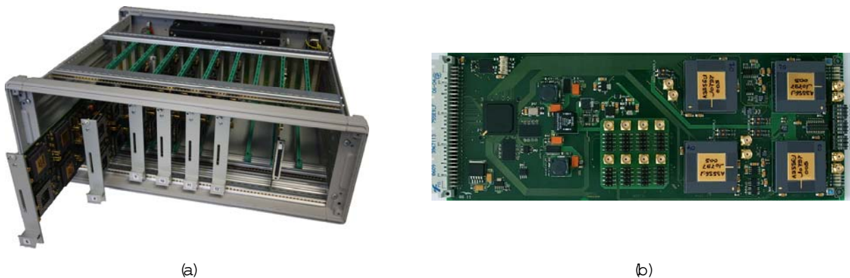
Fig. 3. (a) The global system consists of a rack with a backplane connecting up to 20 boards. Inter-board communication is assured by FPGAs interfacing neurons of a given board to neurons located on other boards. (b) Each board contains 20 neurons spread across 4 analog ASICs, one FPGA, SDRAM memories and additional circuitry used to visualize neurons' membrane potential.
