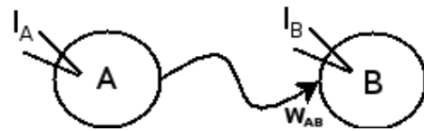
Figure 1: Network of two neurons A and B stimulated by constant currents, respectively I_A and I_B . \omega_{AB} is the synaptic strength of the excitatory synapse connecting A to B.
